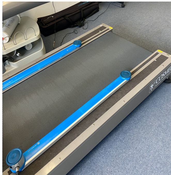
Figure 1: Optogait sensors set up on both sides of the treadmill during testing session two.
